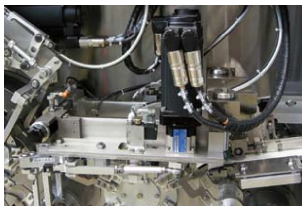
Highly dynamic servomotors for extremely short start/stop cycles
